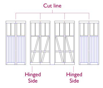
Made from 0.8mm ply (4mm/ft scale) or 1.5ply (7mm/ft scale). Each double door can be cut from its neighbour by running a sharp scalpel blade between each door to cut the tab (shown in red)
